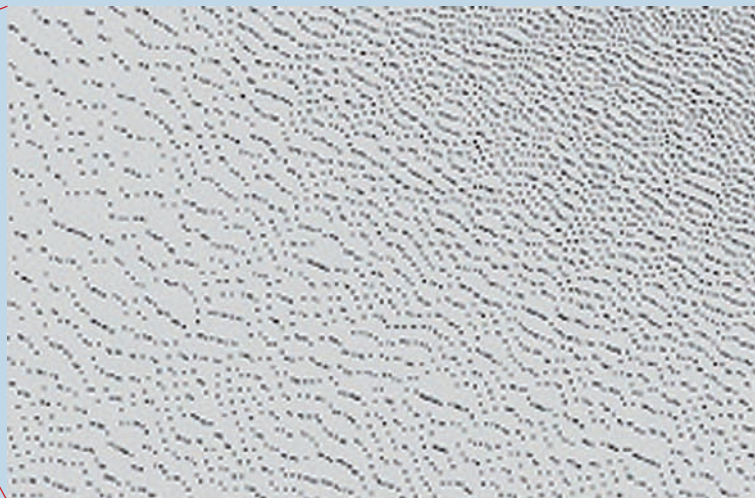
Microscopic view of a Digital Neutral Density Filter with metal micro absorbers.
